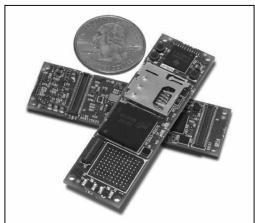
Gumstix Overo COM, a tiny, OMAP-based embedded computer-on-module with Wifi and Bluetooth.
